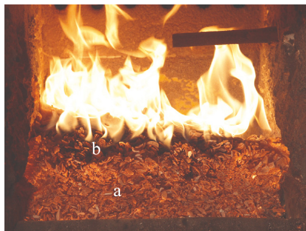
Fig. 8 – Picture of the cross section of the bed 0.45 m (45% of grate length) downstream of the fuel inlet (a. char, b. dry fuel).
