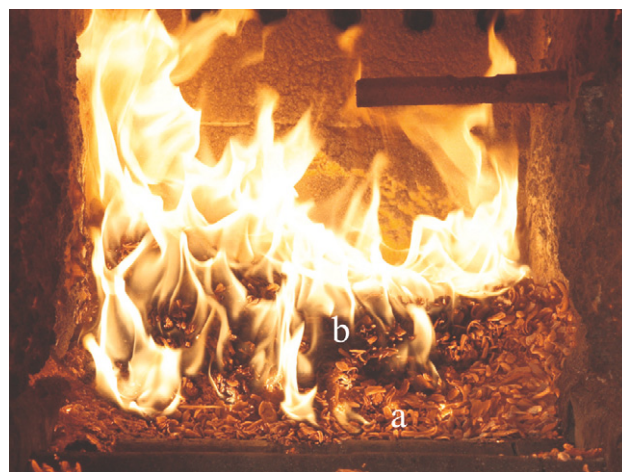
Fig. 9 – Picture of the cross section of the bed 0.3 m (30% of grate length) downstream of the fuel inlet (a. char, b. dry fuel).
